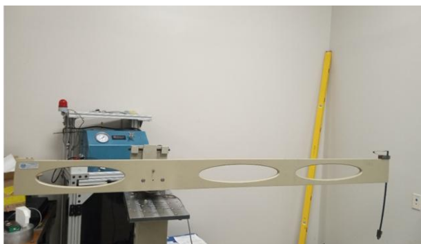
Figure 3. A single-ended unsupported torque arm on a torque cell. The weight of the arm acts at its center of gravity, producing a side load and an overturning moment about the transducer's measurement plane before any calibration weights are applied. From the Morehouse technical paper, Quantifying Overhung Load in Torque Calibration.
