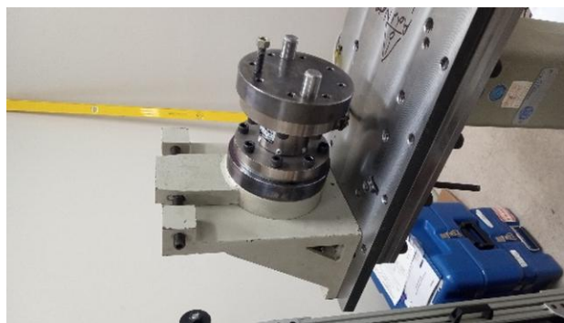
Figure 3. A single-ended unsupported torque arm on a torque cell. The weight of the arm acts at its center of gravity, producing a side load and an overturning moment about the transducer's measurement plane before any calibration weights are applied. From the Morehouse technical paper, Quantifying Overhung Load in Torque Calibration.
