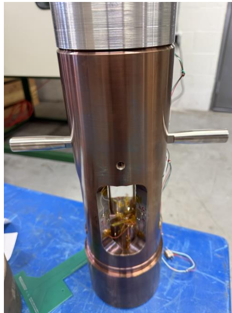
Figure 3. Trimming the gauging on a custom load cell in-house. Adjusting the gauging is one step we use that can drastically improve reproducibility.
