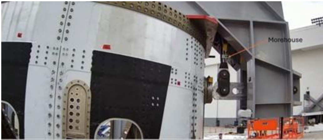
Figure 4. A Morehouse custom load cell was installed in a structural load test.
