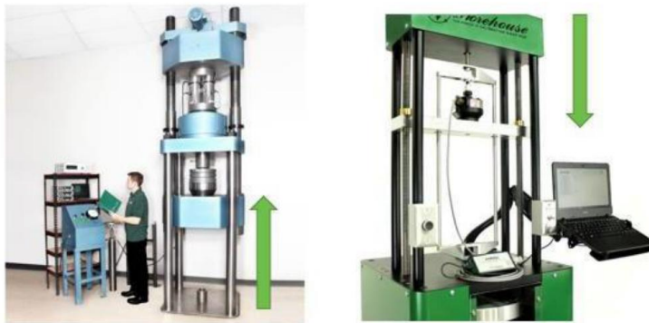
Figure 1. Compression — the load cell is pushed.
