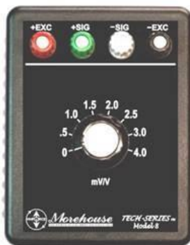
Figure 4. A budget mV/V load cell simulator, 0.5 mV/V to 4 mV/V. Excellent for checks, not adequate for meter substitution.
