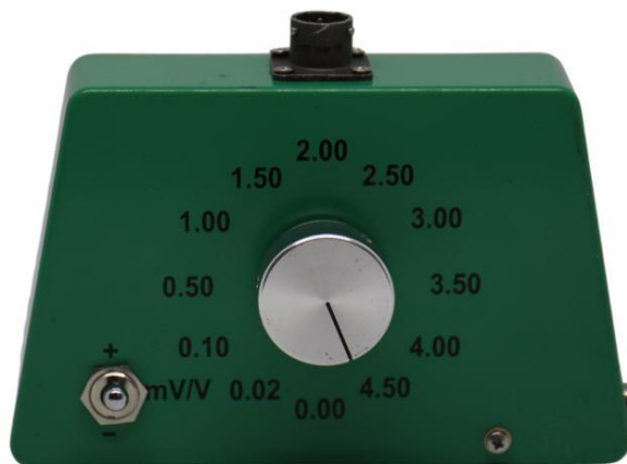
Figure 5. A high-end load cell simulator starting near 0.02 mV/V, low enough to support compliant substitution for many cells.
