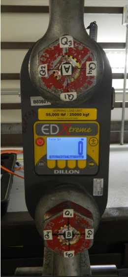
Test setup: B03601 dynamometer with Pin A (top) and Pin B (bottom), each marked into Q1–Q4 quadrants
