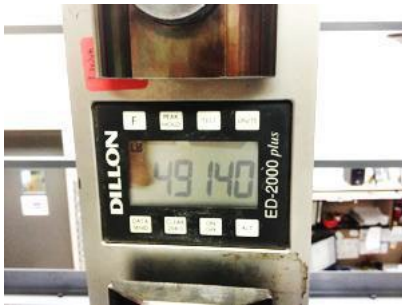
Wrong pin diameter: 49 140 lbf indicated
