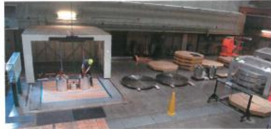
Several of the AF deadweight masses sit on the right, waiting to be calibrated. The balance and measurement station are on the left. Credit: NIST.
