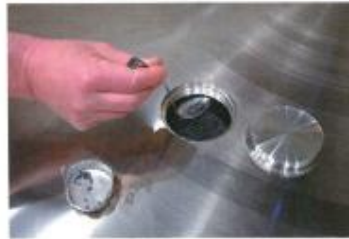
When a mass is too light, NIST staff add small weights into built-in adjustment cavities, that are then sealed up and the mass is re-calibrated. Credit: NIST.
