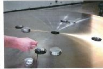
When a mass is too light, NIST staff add small weights into built-in adjustment cavities, that are then sealed up and the mass is re-calibrated. Credit: NIST.
