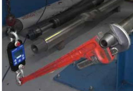
A large display and an audible alarm let workers know when the optimal torque has been reached.
