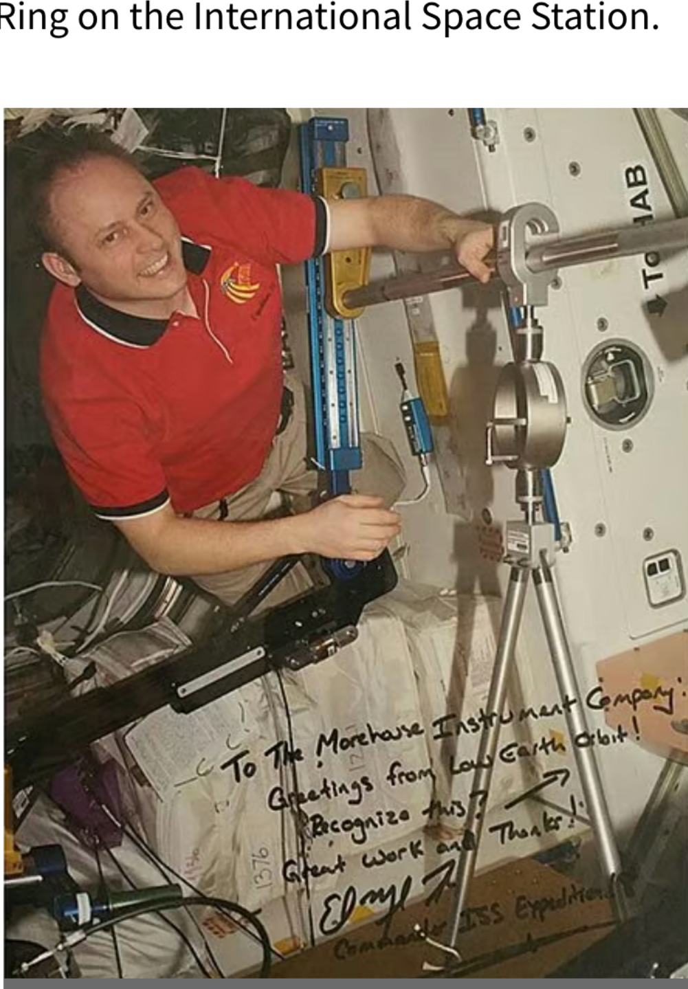
Figure 8: A Morehouse Proving Ring being used on the International Space Station
