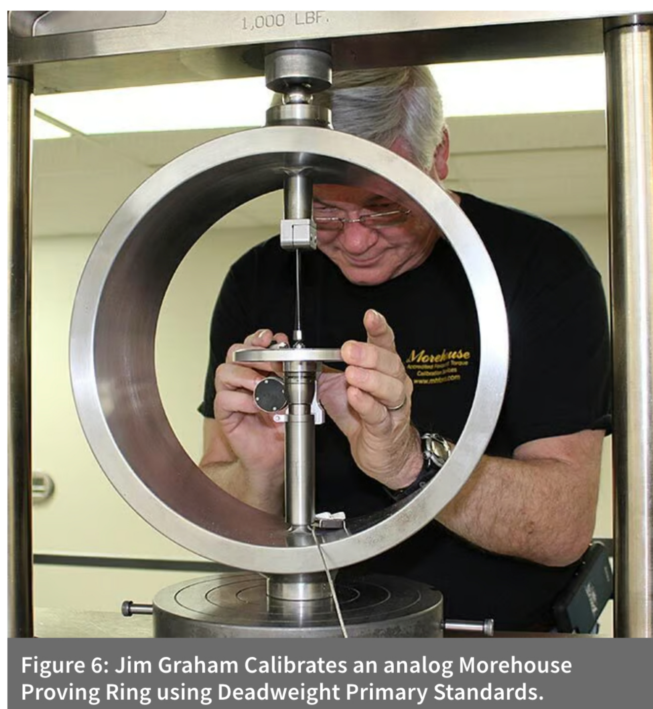
Figure 6: Jim Graham Calibrates an analog Morehouse Proving Ring using Deadweight Primary Standards.
