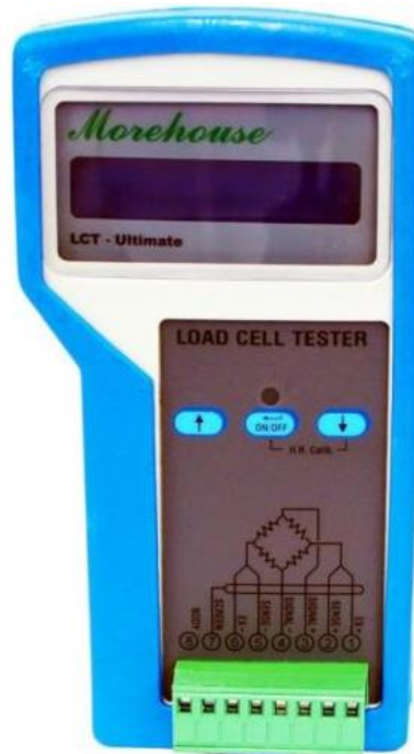
Figure 8 A Morehouse Load Cell Tester
