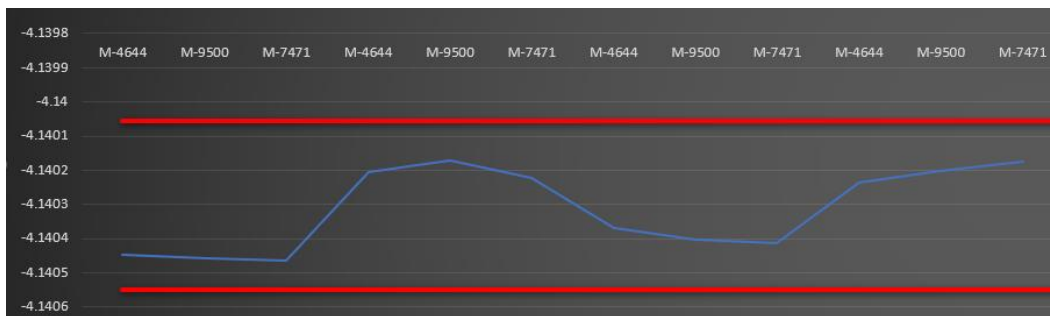
Figure 9: A Control Chart Comparing the mV/V Output of One Load Cell in Three Different Deadweight Force Machines Over Time
