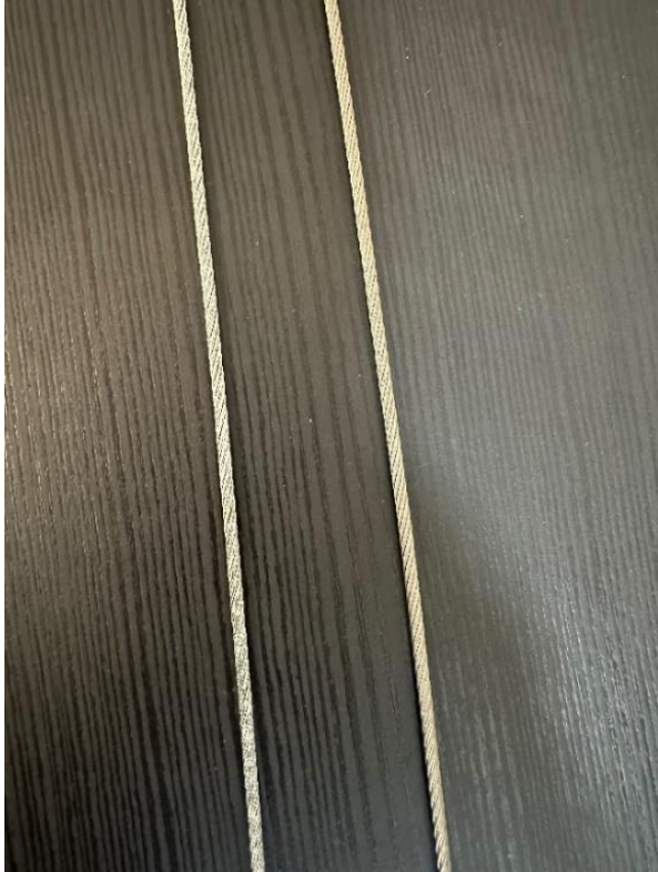
Two 3/32" Cables. The one on the left is a GAC, and the other an SSAC
