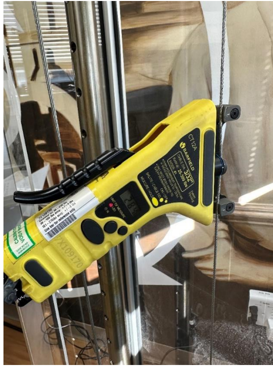
Figure 1: Barfield Digital CT12A Cable Tensiometer in the Morehouse PCM-2MD-T1 Cable Tensiometer Calibrator.
