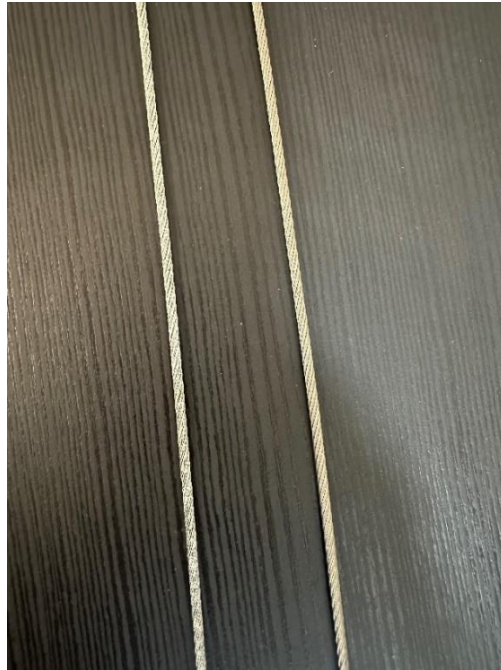
Figure 9: Two 3/32" Cables. The one on the left is a GAC, and the other an SSAC.
