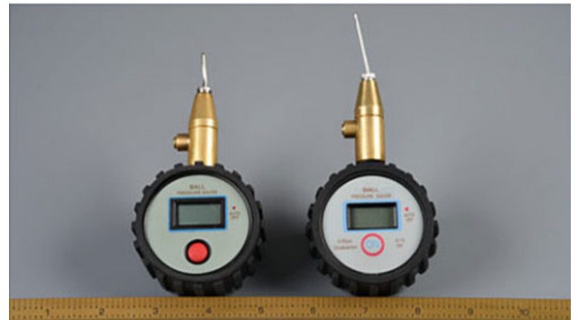
Figure 6 Pressure Gauges used by the championship officials to measure internal air pressure at halftime. (Exponent 2015) 3
