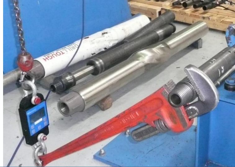
A large display and an audible alarm let workers know when the optimal torque has been reached.
