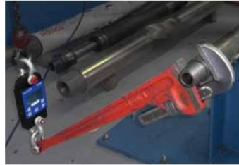
A large display and an audible alarm let workers know when the optimal torque has been reached.
