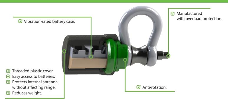
Our shackle load pins outperform others on average by a typical 10:1 performance margin and boast a robust 5x overload capacity and superior IP67 protection. With wireless capabilities, these pins allow monitoring from a 600-meter range, enhancing safety and operational efficiency across various lifting and rigging tasks.
