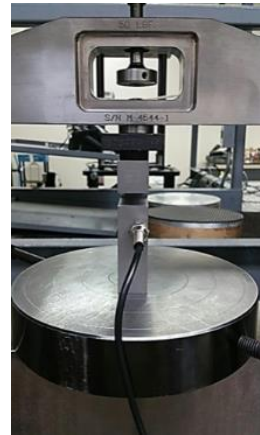
S-BEAM WITH 0.75 % MISALIGNMENT ERROR VS MOREHOUSE WITH 0.0022 % ERROR
