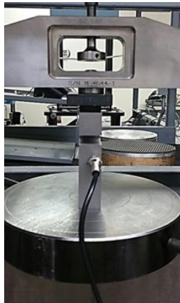
S-BEAM WITH 0.75 % MISALIGNMENT ERROR VS MOREHOUSE WITH 0.0022 % ERROR
