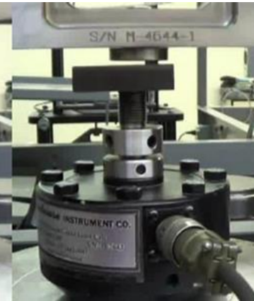
S-BEAM WITH 0.75 % MISALIGNMENT ERROR VS MOREHOUSE WITH 0.0022 % ERROR
