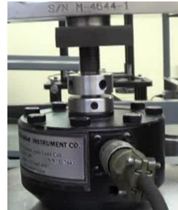
S-BEAM WITH 0.75 % MISALIGNMENT ERROR VS MOREHOUSE WITH 0.0022 % ERROR
