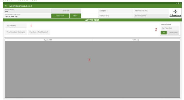
The active test screen displays the current UUT readings (1), the state of the system, and results from past and ongoing calibration runs (3). It also contains controls for a manual run (2).
