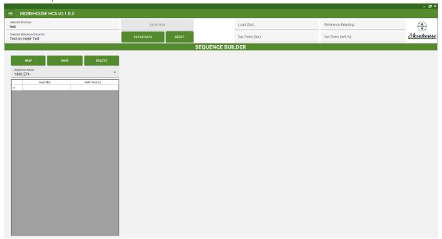
The Sequence Builder screen allows the user to create sequences that can be called up later to perform a calibration. An existing sequence can be modified by selecting it from the dropdown, making the required changes, and pressing save. It can also be deleted by pressing delete. A new sequence can be created by pressing new, entering the desired name, and pressing ok. Make sure the new sequence is selected from the drop-down before making changes and pressing save.
