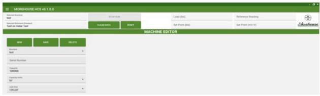
The Machine Editor screen allows the user to enter the parameters for machines (UCM or USC) that the system will be connected to.
