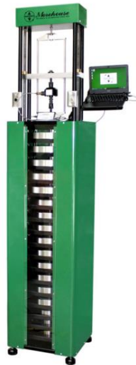
Figure 11 Morehouse 1,000 lbf automated deadweight machine
