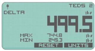
Soft keys allow to Reset the min and max to the current value. i.e. zero the Delta. The usual Units selection is also available.
