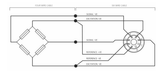
Where Strain Bridge Sensor Chassis is Metallic (or surrounding strain bridge sensor structure)
