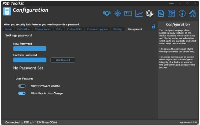
Access to the entire set of Configuration settings can be locked with a password. Without the password a user cannot change any of the protected settings which include the available Display Modes.
