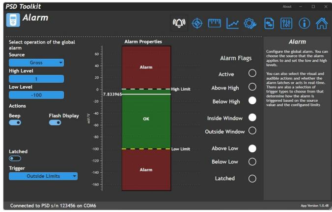
The single, global alarm acts on the currently selected calibration range (or TEDS device) and is solely based on the Source selected here.
