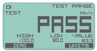
The High limit, Low limit and actual Value are displayed underneath. Soft keys allow for toggling between Zero and Gross and the Units can be selected.
