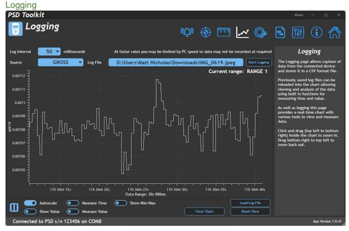
This page allows data from the handheld to be logged to a file and later reloaded to be viewed on the chart. A real-time chart is always visible whether logging is active or not.
