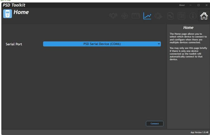
When you connect the handheld to the PC using a USB cable it creates a virtual COM port on the PC. All detected PSD devices are displayed in the drop-down list and you need to select the appropriate one. If only one handheld is detected you may not see this page as the Toolkit will automatically select and connect to it.
