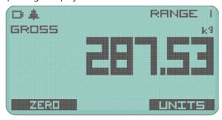
The current calibration range is display top right and Gross or Net is displayed above the main value. Current units are displayed above right of the main value.
