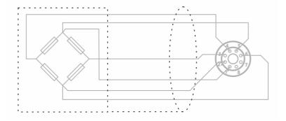
Where There is No Option to Connect to Strain Bridge Sensor Chassis
