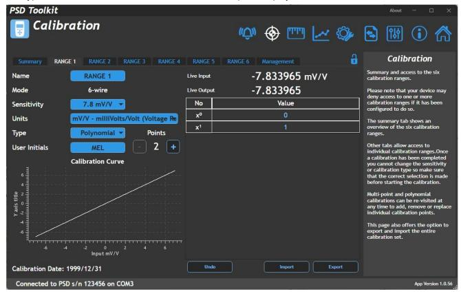
Polynomial calibration allows linearization of up to 11 points. Note that you must use the Points [+] button to add one point at a time. Once the polynomial value has been entered the button will be enabled to allow another point to be added.
