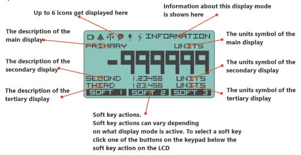
The **values** for the main, secondary and tertiary items are not indicated on the above diagram to improve clarity.
