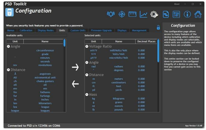
This section allows you to define which units of measure are available for calibration as the base engineering units and also any unit conversions that are selectable from the Units soft key that appears on most display modes. Two lists are displayed. The left one shows all available units that are *not* currently enabled and the one on the right shows the units that are available for calibrating or conversion.
