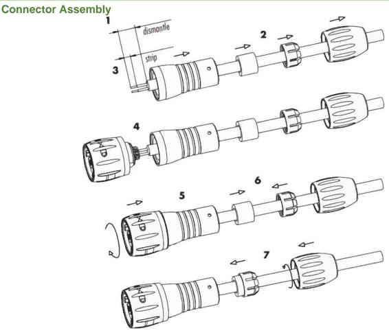
If a cable is already connected to the connector remember to unscrew the cable clamp before unscrewing the main body of the connector otherwise, you risk twisting the cable and breaking the connections. If the main body is difficult to unscrew it may be easier to lock the connector to the handheld then grip and unscrew the main body in an anti-clockwise direction.
