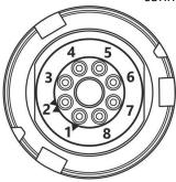
View from solder connector side of the connector
