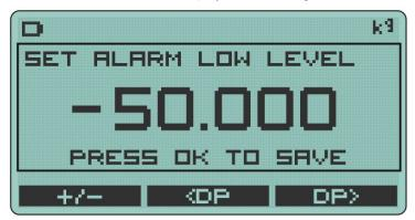
The text at the top right states the engineering units of the value being entered. The text at the top inside the box states what parameter is currently being edited.
