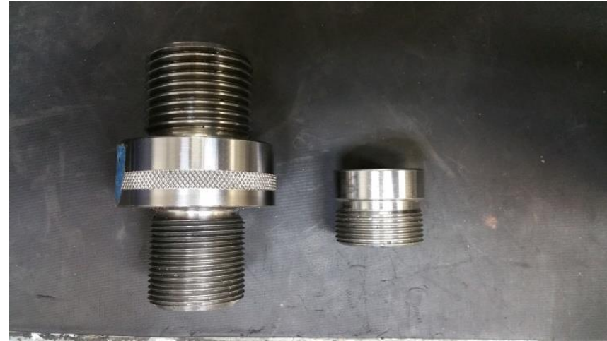
Different type adapters. (1.5" engagement versus 0.5 " engagement)
