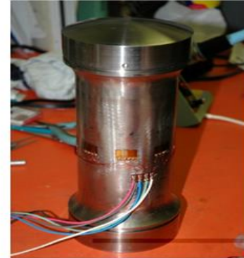
Wired Wheatstone bridge of load cell.
