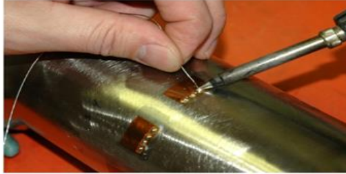
Tinning of strain-gage solder tabs.
