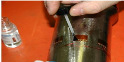
Removing excess soldering flux.
