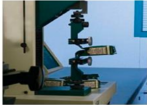
Fig 11. Testing the strength of coffee packaging using the quick release vise grips, HT55
