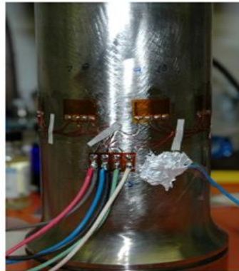
Ground wire added.
