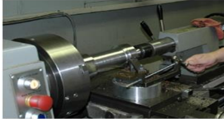
Machining of Viscount 44 bar stock.
