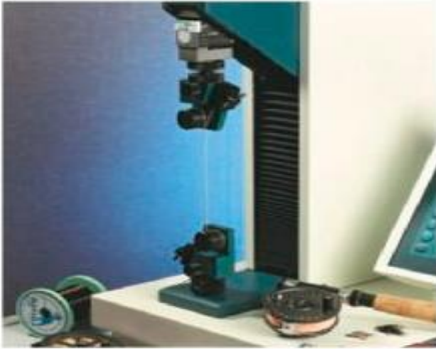
Fig 12. Testing the strength of fishing line using single bollard grips, HT33
