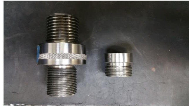
Different type adapters. (1.5" engagement versus 0.5 " engagement)
