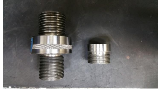
Different type adapters. (1.5" engagement versus 0.5 " engagement)
