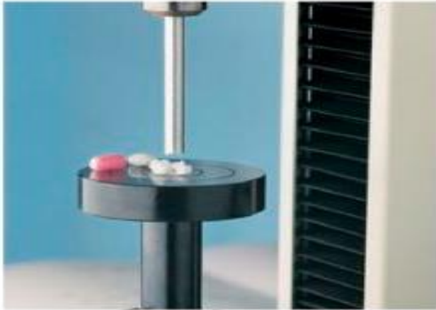
Fig 15. Testing the crushing strength of pills
