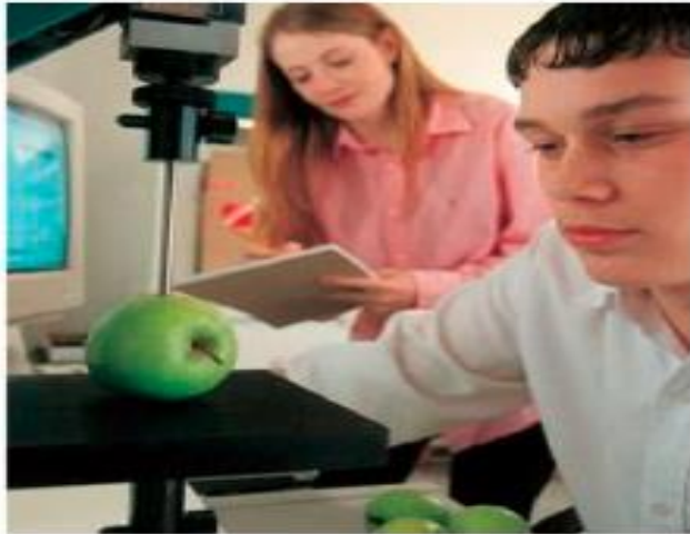
Fig 10. Testing the ripeness of apples using a set of Magnus Taylor probes
