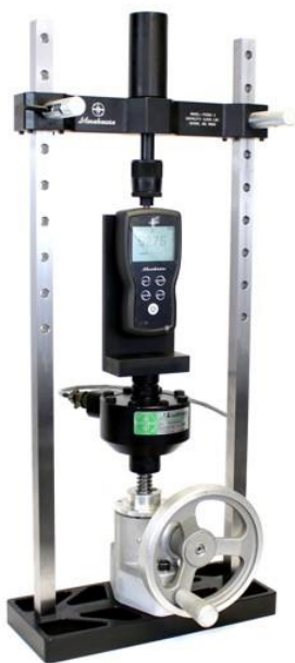
Figure 92: An Example of Low Torsion Using a Morehouse Portable Calibrating Machine
