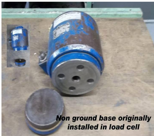
Figure 108: Multi-Column 300K Load Cell with a Non-Ground Base
