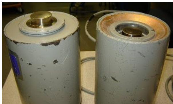
Figure 32: Overloaded Load Cell
