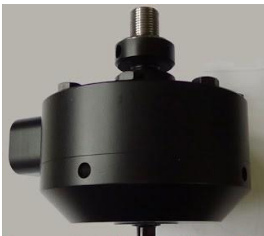
Figure 116: Improper Way to Thread an Alignment Plug: Thread is Not Engaged Enough into the Load Cell
