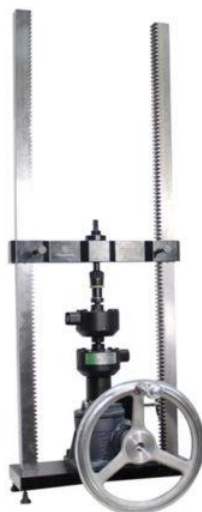
Figure 90: An Example of Square Using a Morehouse BCM
