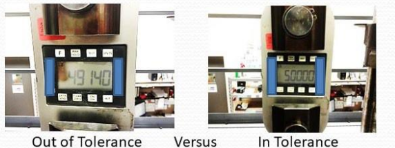
Figure 120: Tension Link Difference in Output with Pin Size
