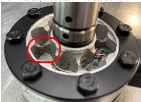
Figure 34: Inside of an Overloaded Shear Web Load Cell Showing a Clear Break of the Web Element
