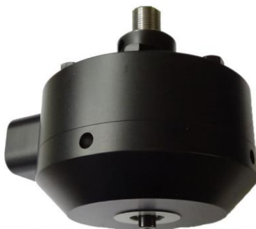
Figure 115: Proper Way to Thread an Alignment Plug: Thread is Past Flush and Into Cell
