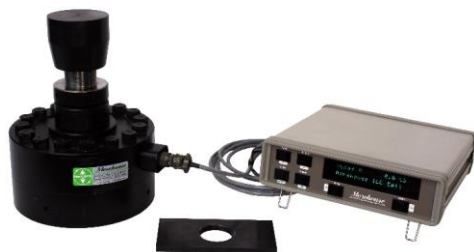
Figure 173: ILC rental kit with 100k load cell and 4215 indicator
