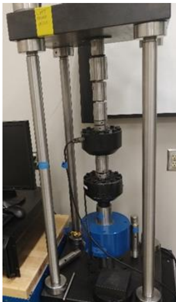
Figure 82 Compression/Tension Machine that Does Not Replicate Field Use
