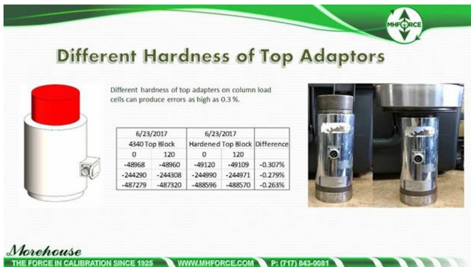
Figure 104: Different Hardness of Top Adaptors
