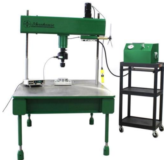
Figure 91: An Example of Rigid Using a Morehouse USC-60K Scale Press
