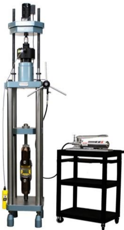
Figure 89: An Example of Level Using a Morehouse UCM
