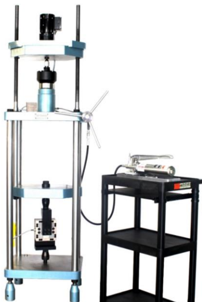
Figure 84 Morehouse Universal Calibrating Machine with a Unit Under Test in Tension using ISO 376 Compliant Tension Adapters
