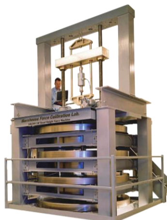
Figure 174: Morehouse 120,000 lbf deadweight machine
