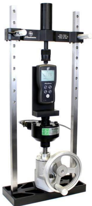
Figure 65: Morehouse 2,000 lbf Portable Calibrating Machine
