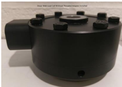
Figure 96: Morehouse Calibration Grade Load Cell Without Integral Threaded Adapter
