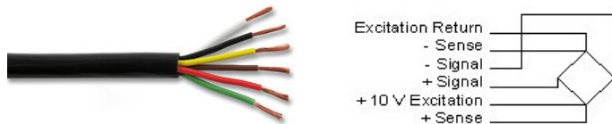
Figure 146: 6-Wire Cable and Diagram
