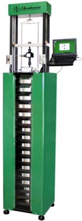
Figure 88: A Morehouse Primary Standard Automated Deadweight Machine
