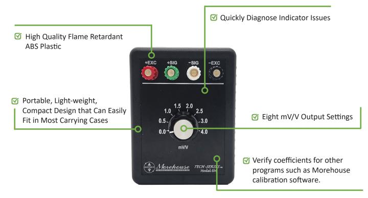
Morehouse portable, lightweight, Model 8 Budget Load Cell Simulator can be a helpful tool in troubleshooting equipment problems; the load cell simulator can be used to verify meters are reading correctly, span meters, and as a check standard to help identify drift associated with many digital meters.
