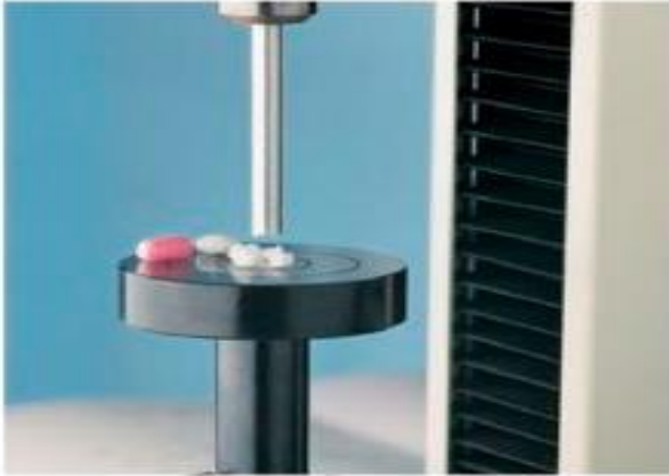
Fig 15. Testing the crushing strength of pills
