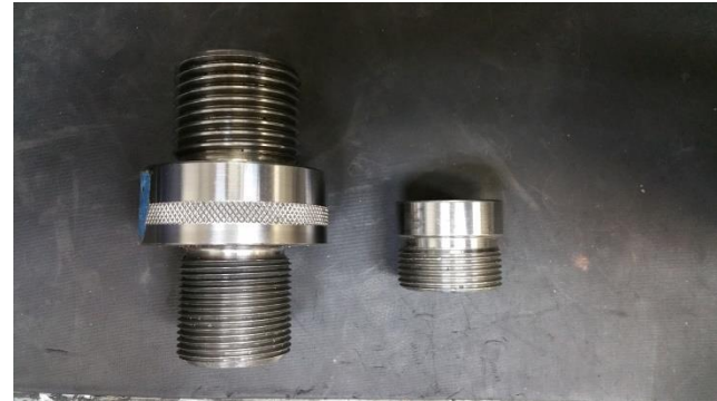
Different type adapters. (1.5" engagement versus 0.5 " engagement)
