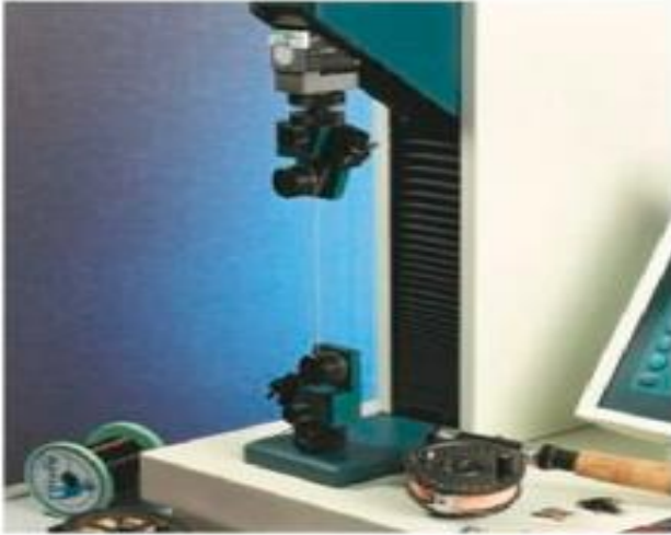
Fig 12. Testing the strength of fishing line using single bollard grips, HT33
