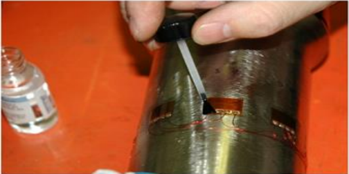
Removing excess soldering flux.
