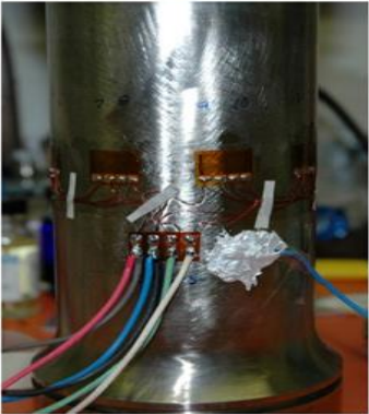
Ground wire added.
