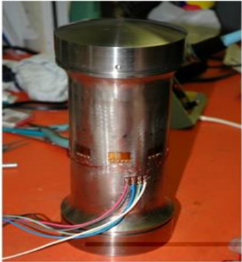
Wired Wheatstone bridge of load cell.
