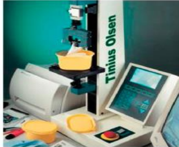
Fig 19. Testing the adhesive peeling forces of foil packaging
