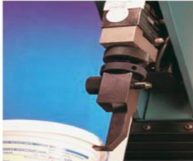
Fig 21. Determining the force to remove the lid from a plastic package
