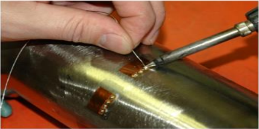
Trimming of strain-gage solder tabs.
