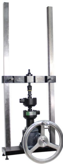
Figure 11. Morehouse BCM Example of Load Cell Calibration
