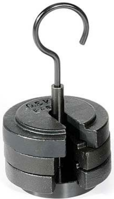
Figure 2. Stacking Weights on a Hook
