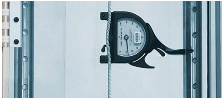
Figure 7. Cable Tensiometer Calibration
