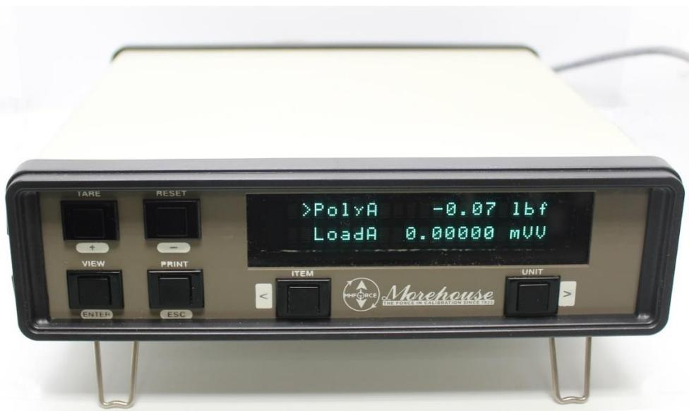
The quickest way to verify that the coefficients have changed is to compare what is read when the indicator is on the PolyA force units, and LoadA mV/V. The PolyA value in force units is the same as the B0 coefficient when the tare button is pressed.
