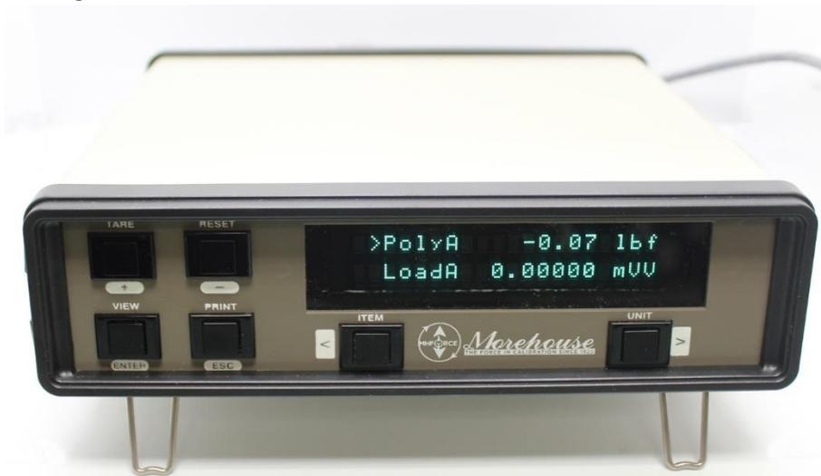
5. Make sure the display is set to use the polynomial formula. To do this one line must be set to **PolyA** and force units and the other line should be set to **LoadA mV/V**. This is done by using the
