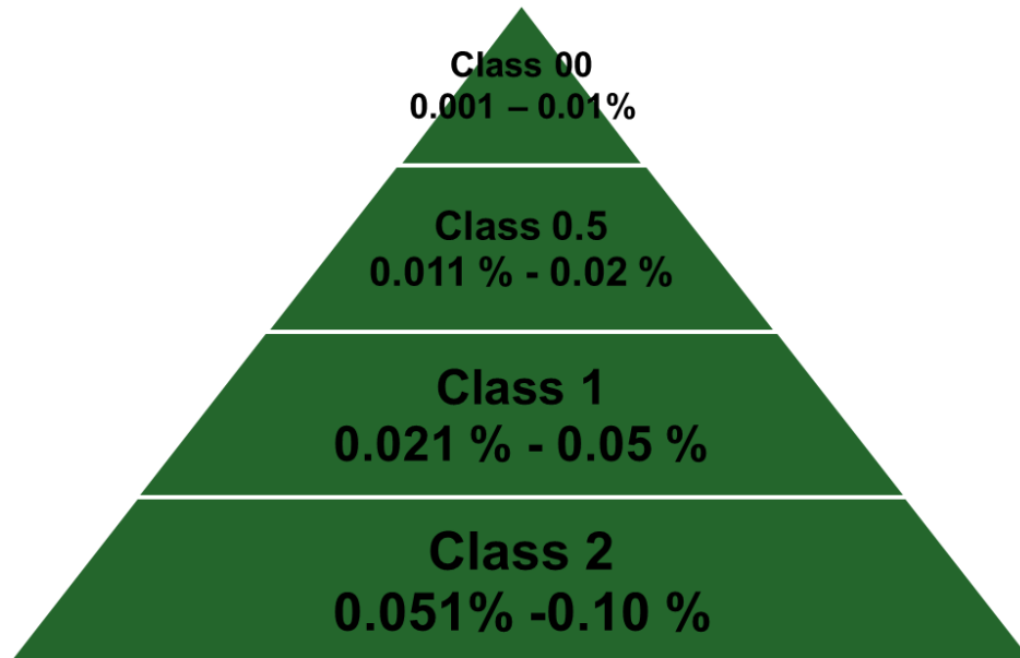
Figure 1: ISO 376 Expanded Uncertainty Required to Classify a Force-Proving Instrument
