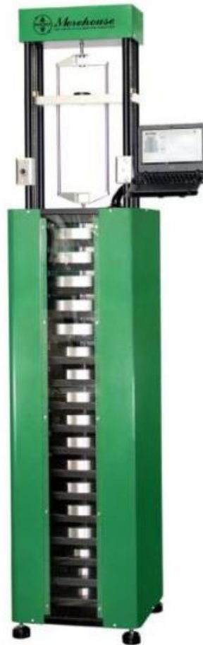
Figure 9: Morehouse Deadweight Machine
