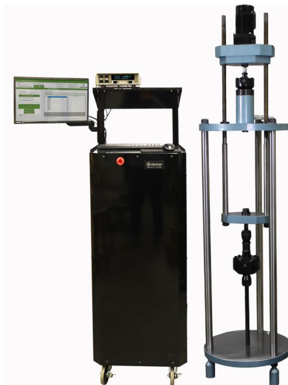
Figure 4: A Morehouse 30K Automation Setup.
