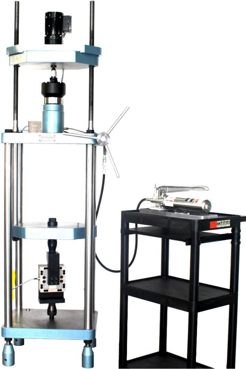
Figure 1: A Morehouse UCM with a Device Under Test (DUT) In Tension Using ISO 376 Compliant Tension Adapters
