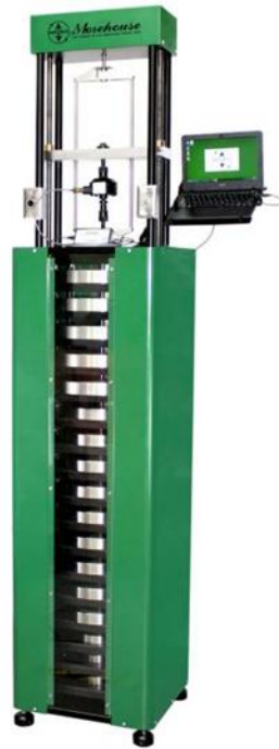
Figure 11 A Morehouse Deadweight Calibration Machine
