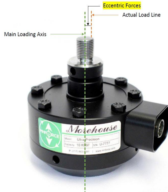
Figure 10 A Morehouse Load Cell Showing What Eccentric Forces Are
