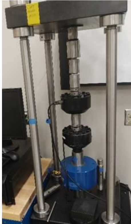
Figure 16 Picture of a Compression/Tension Machine that Does Not Replicate Field Use
