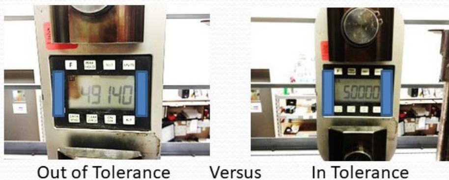
Figure 1 Tension Link Difference in Output with Pin Size
