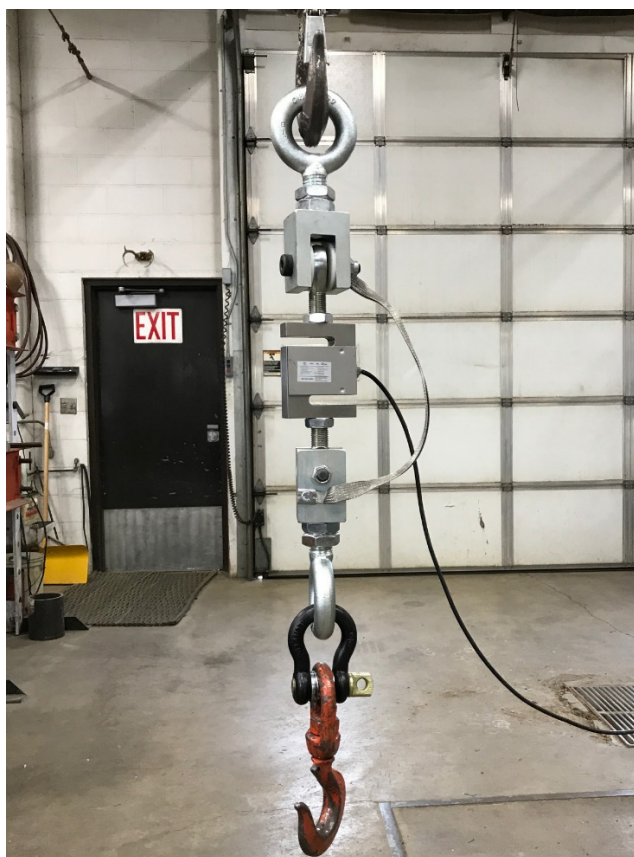
Figure 3 S-Beam Load Cell with Six Adapters
