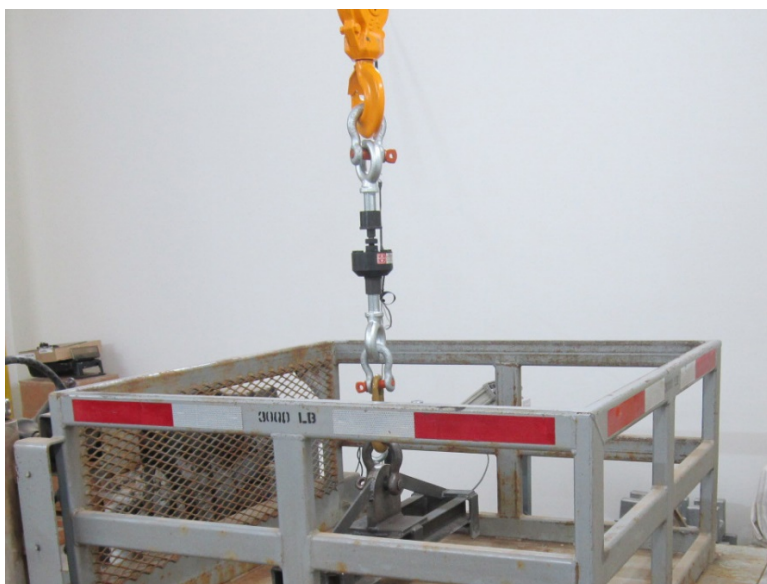
Figure 4 Morehouse Precision Calibration Load Cell with Custom Adapters
