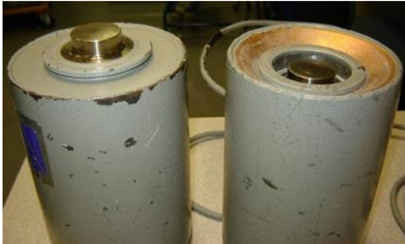
Figure 2: Overloaded Load Cell
