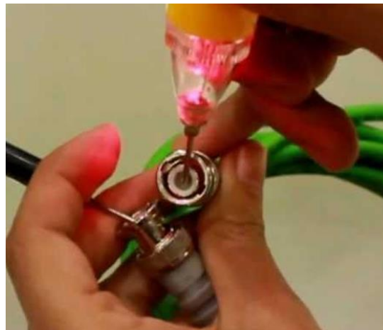
Figure 5: Checking for Continuity of the Cable
