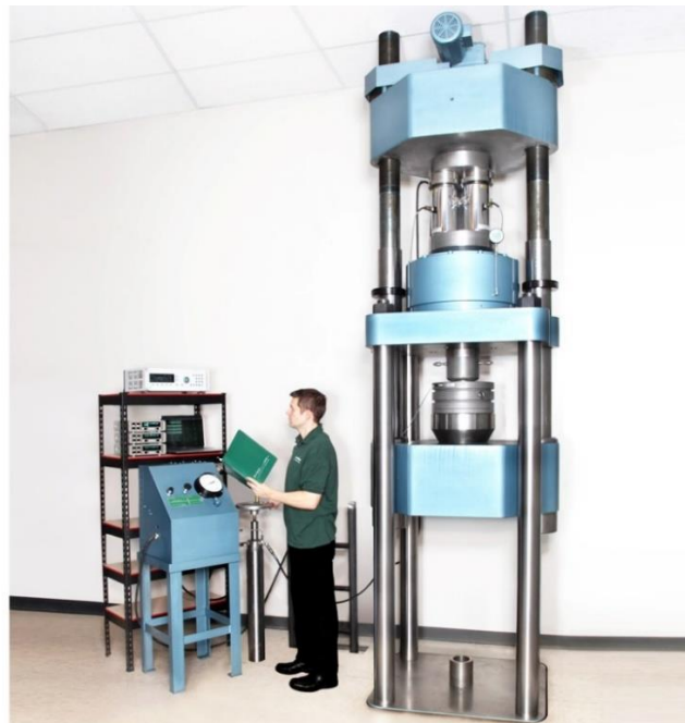
Figure 1: Morehouse Universal Calibrating Machine (UCM)
