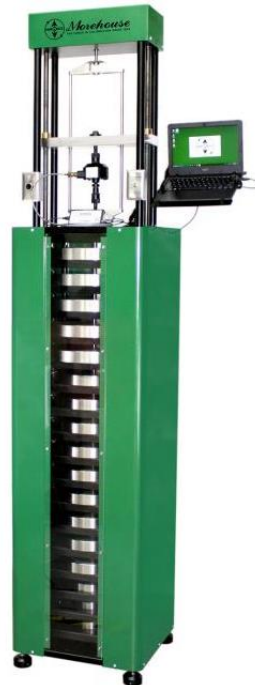
Figure 7: Morehouse Primary Standard Deadweight Calibrating Machine (DCM)
