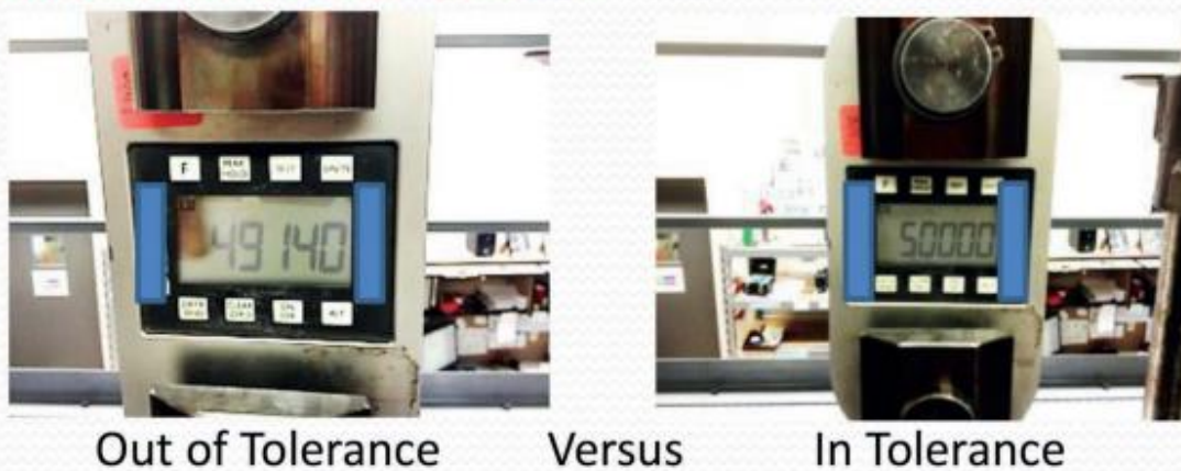
Figure 4: Tension Link Loaded into a Morehouse Deadweight Machine with Accuracy of Better than 0.002 % of the Applied Force
