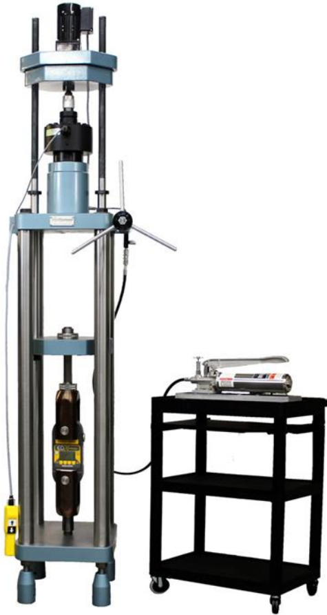
Figure 8: Morehouse Universal Calibrating Machine (UCM)
