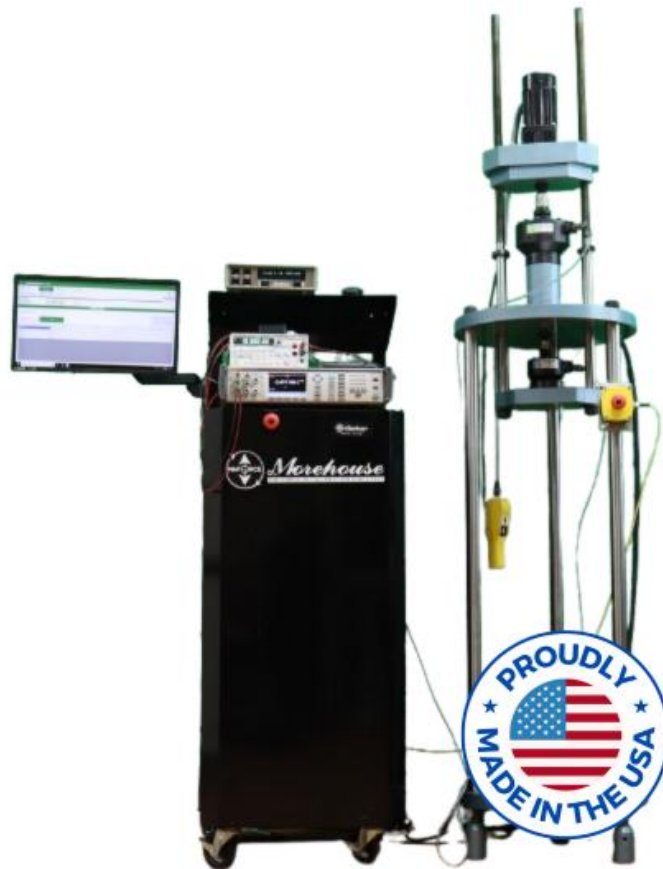
Figure 9: Morehouse 30k UCM with Automation Upgrade
