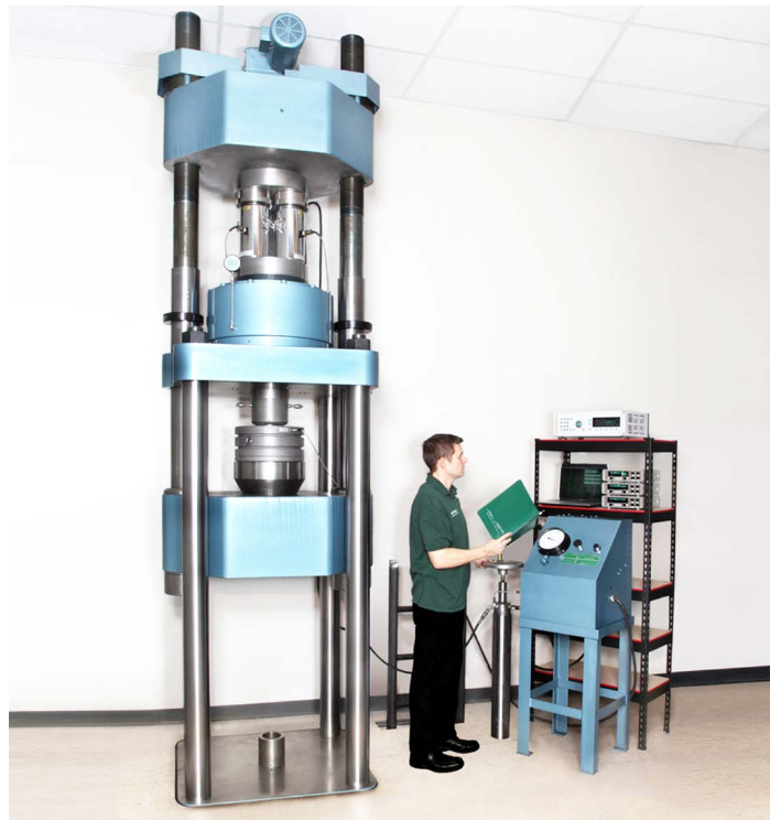
Figure 3: Reference Standard Calibration with Morehouse Secondary Standard
