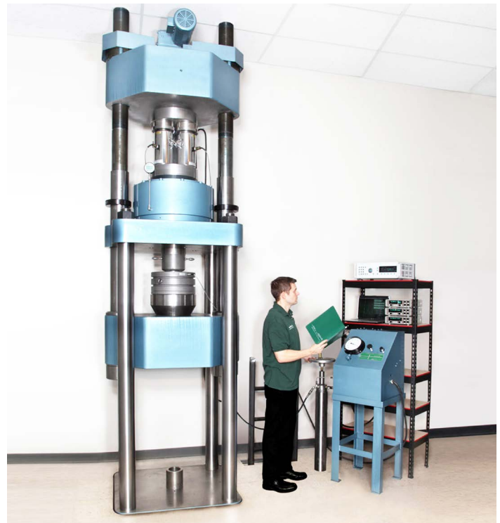
Figure 3: Reference Standard Calibration with Morehouse Secondary Standard
