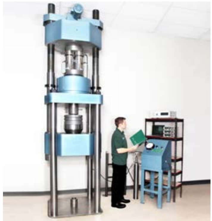
Figure 3: Reference Standard Calibration with Morehouse Secondary Standard
