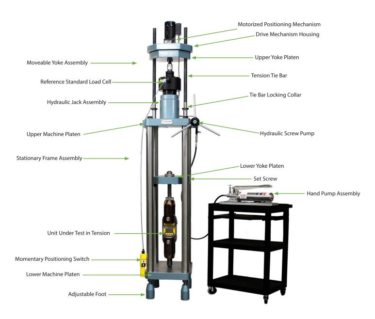
Figure 3: Morehouse Universal Calibrating Machine 100,000 lbf (500 kN) Capacity (with motorized adjustable yoke platen)
