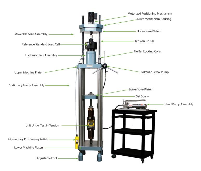
Figure 11: Morehouse Universal Calibrating Machine 100,000 lbf (500 kN) Capacity (with motorized adjustable yoke platen)
