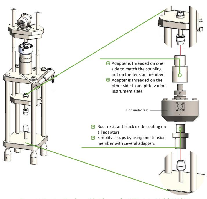
Figure 20: Tension Members with Adapters for UCMs 100,000 lbf (500 kN)
