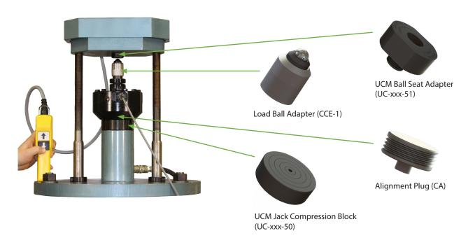
**Figure 9: Reference Standard Setup and Adapters**
