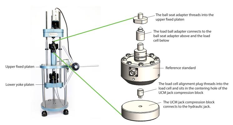
Figure 8: Reference Standard Kit for Capacities 100,000 lbf (500 kN) and Lower
