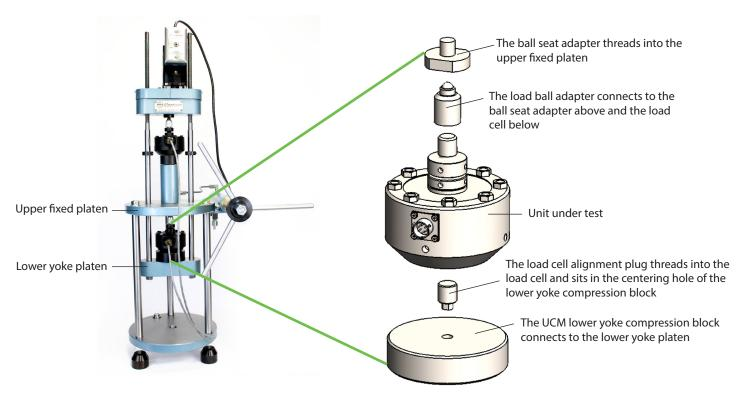
**Figure 18: Setup for Compression Calibration**
