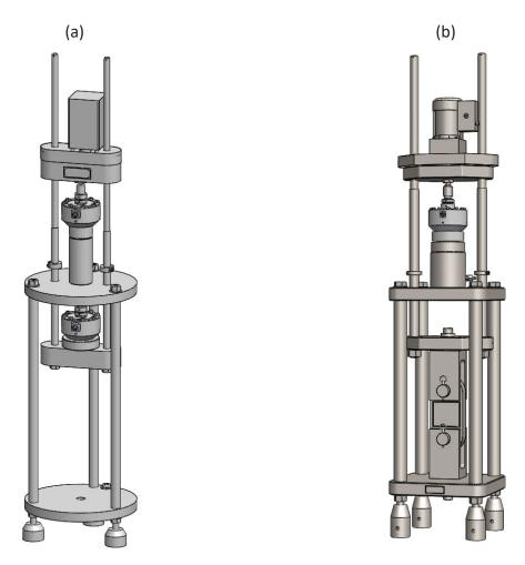
Figure 15: Calibrating Instruments in a) Compression; b) Tension
