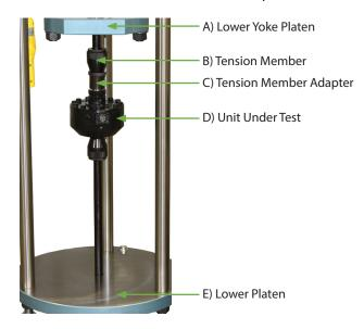
**Figure 24: Tension Member Setup**
