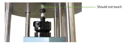
Figure 17: Unit Under Test Clearance
