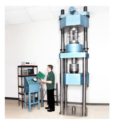
Figure 1: Morehouse Universal Calibrating Machine 1,000,000 lbf Capacity
