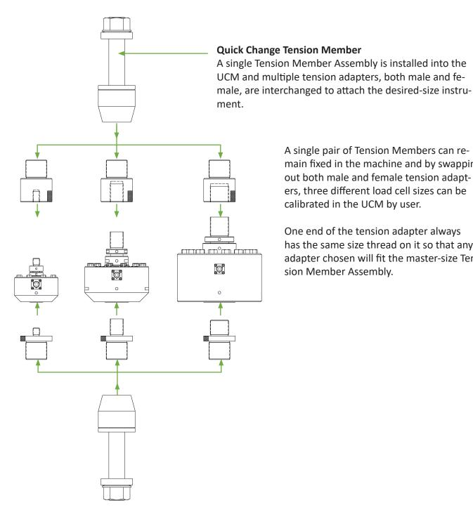
A single pair of Tension Members can remain fixed in the machine and by swapping out both male and female tension adapters, three different load cell sizes can be calibrated in the UCM by user.
