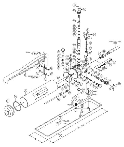
Figure 25: Hand Pump Assembly (Drawing 214000A-01)
