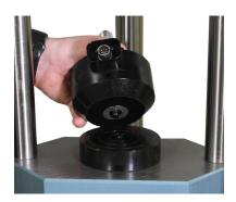
Figure 16: Unit Under Test with Alignment Plug
