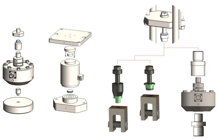
Figure 26: Adapters for the Universal Calibrating Machine
