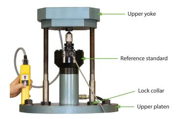
**Figure 12: Reference Standard Setup**
