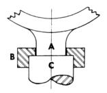
Figure 13: Proving Ring Adapters
