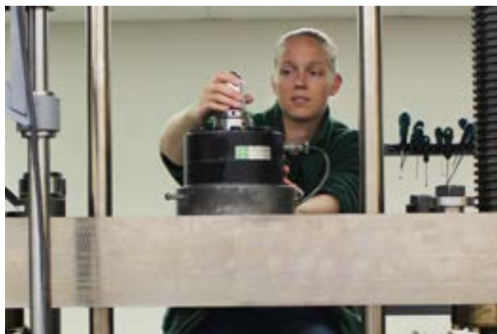
Figure 2: Reference Standard Calibration with Morehouse Primary Deadweight
