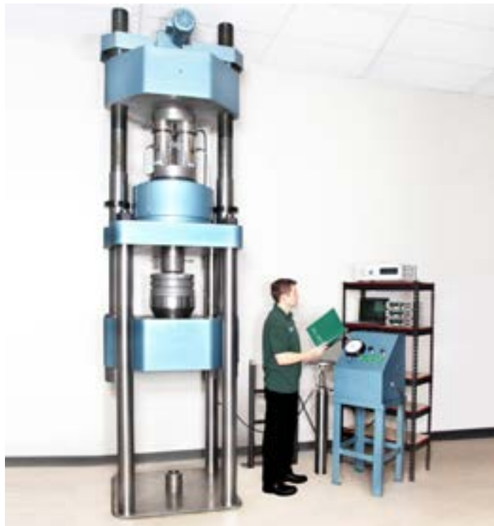
Figure 3: Reference Standard Calibration with Morehouse Secondary Standard
