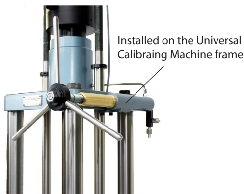
Auxiliary Screw Pump used with a Hydraulic Hand Pump
