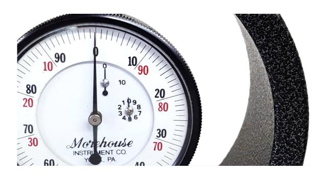
Note: Expanded Scale indicators are not direct reading.
