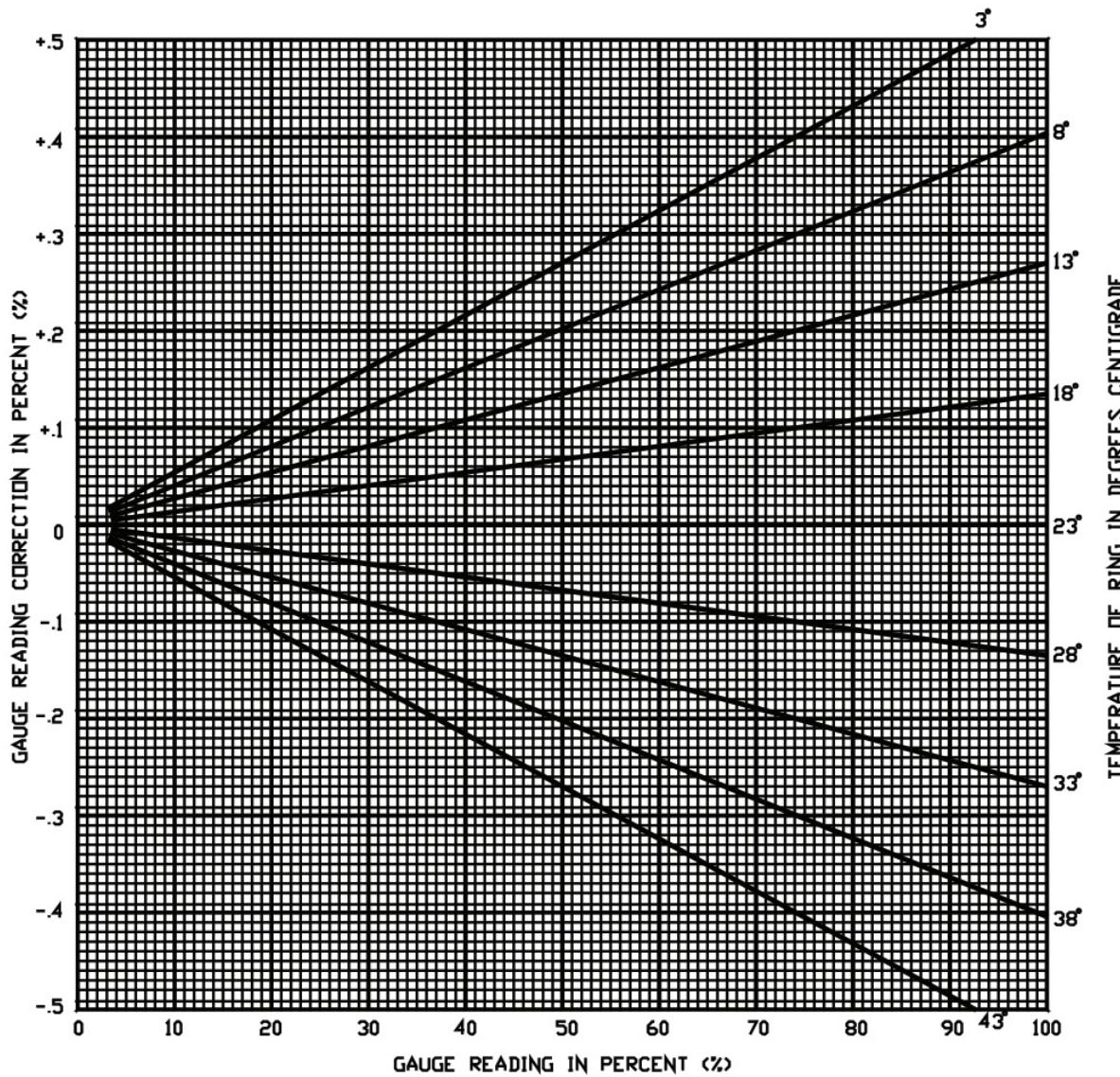
**Figure 3: Temperature Correction for Centigrade Scale (Drawing 99332-1)**
