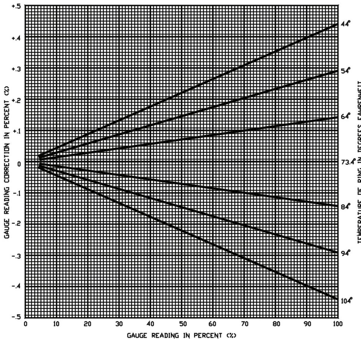
**Figure 2: Temperature Correction for Fahrenheit Scale (Drawing 99332)**
