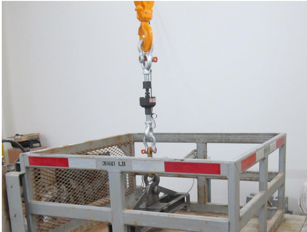
Morehouse Precision Calibration Load Cell with Custom Adapters
