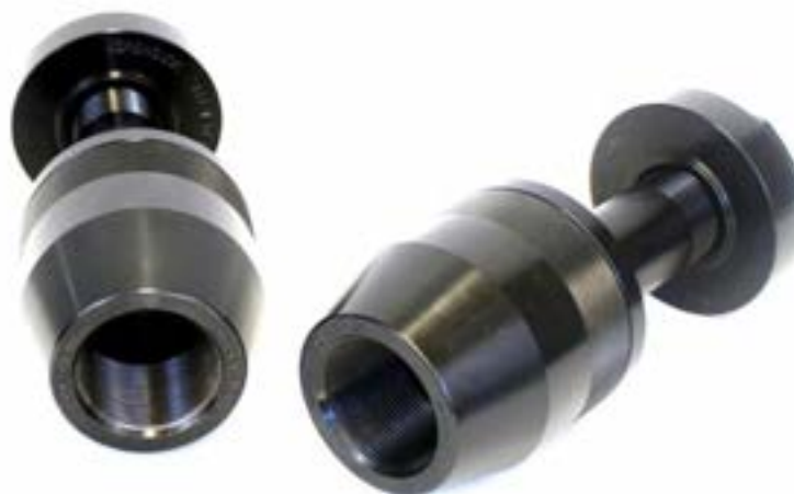
Figure 3: Set of 120,000 LBF Tension Members
