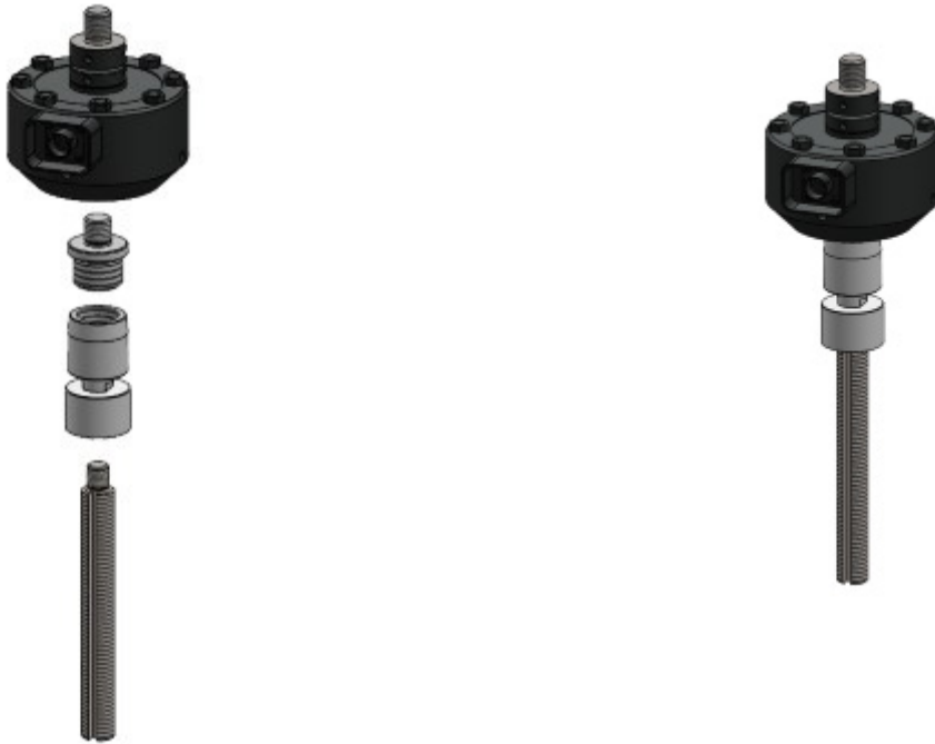
Figure 3: Installation of Reference Load Cell Using the Standard Mounting Adapter
