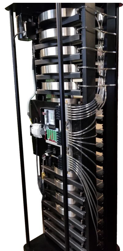
Figure 10: Pneumatic System Removes or Applies Weights
