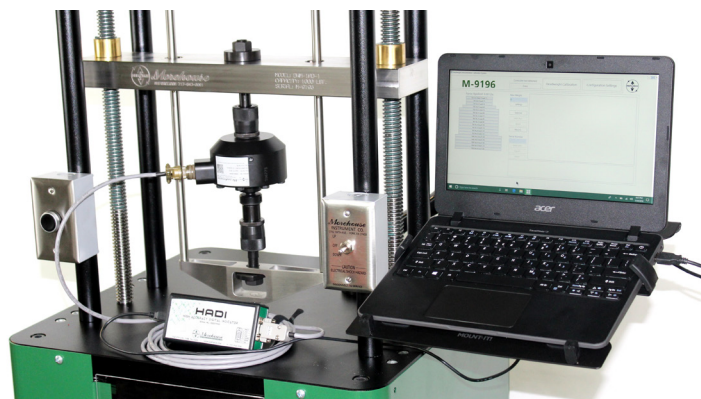
Figure 8: Control and Automate with the Deadweight Calibration System (DCS)
