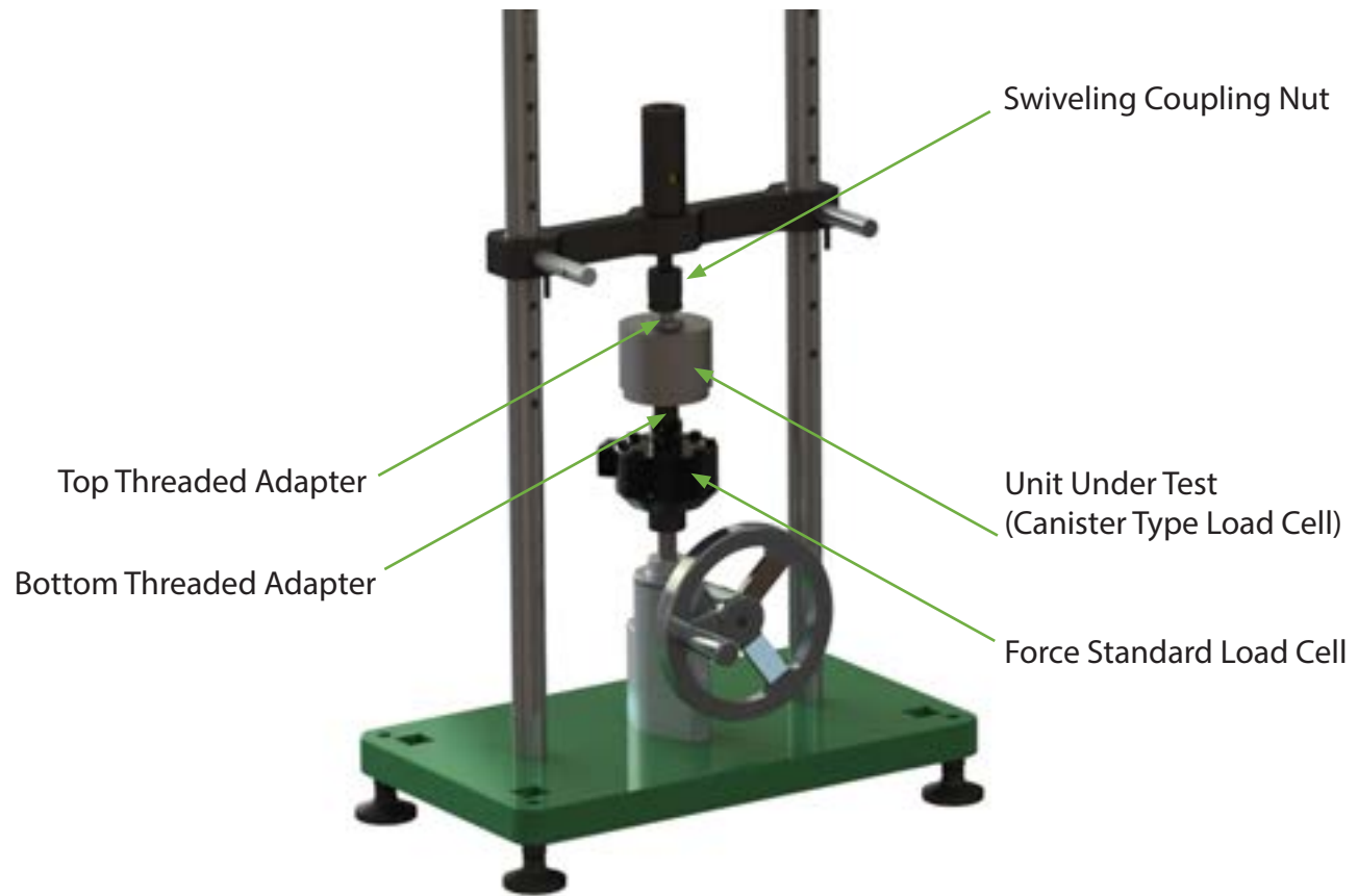
Figure 5: Tension Calibration Setup Using Threaded Adapters (Safety Shield Not Shown for Better Demonstration of the Setup)
