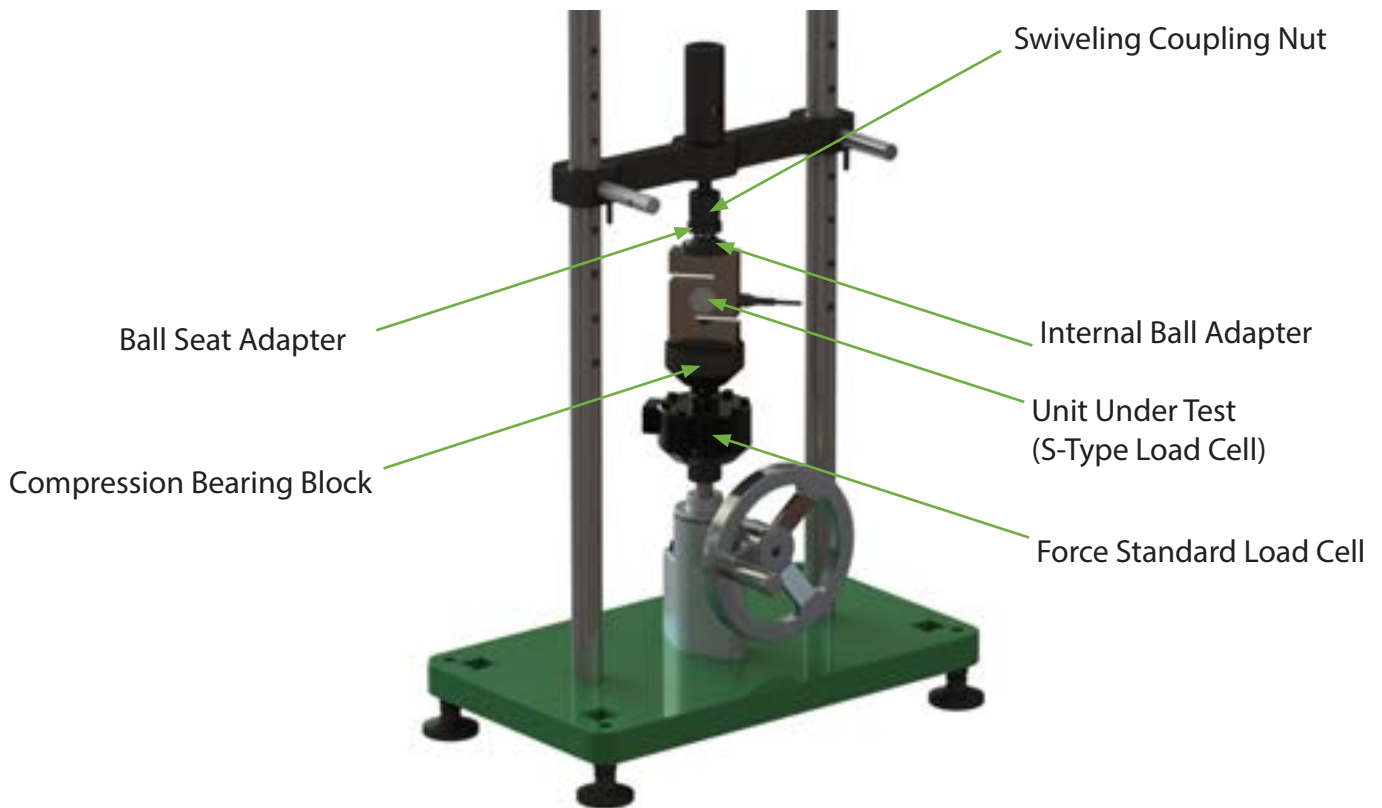
Figure 7: Compression Calibration Setup Using Internal Ball Adapter (Safety Shield Not Shown for Better Demonstration of the Setup)
