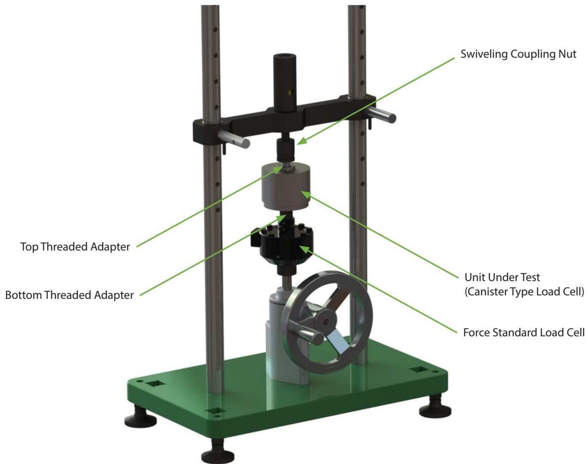
Figure 5: Tension Calibration Setup Using Threaded Adapters (Safety Shield not Shown)
