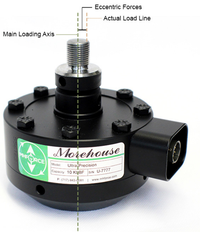
Figure 11: Load Cell Showing Eccentric Forces
