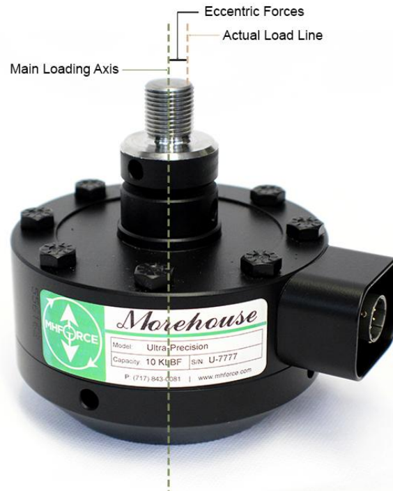
Figure 2: Load Cell showing eccentric forces
