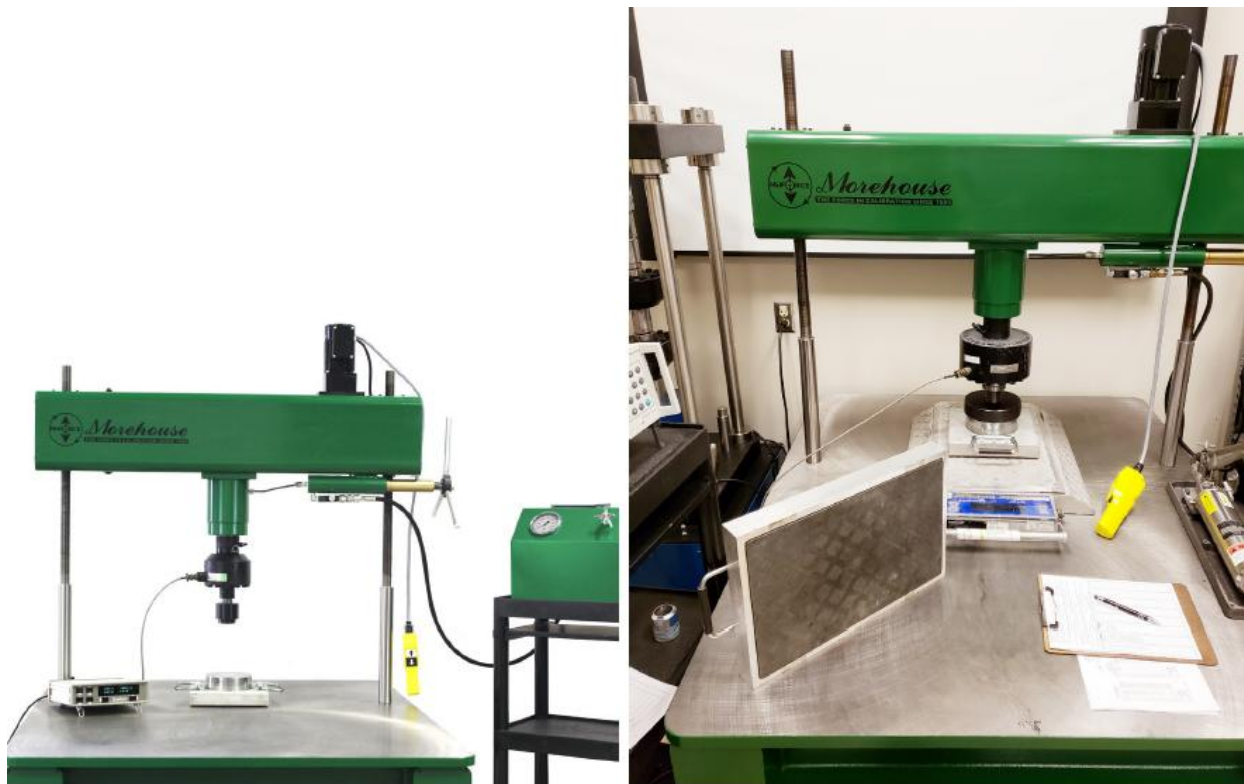
Figure 14: Calibration Adapter for Truck and Aircraft Scales
