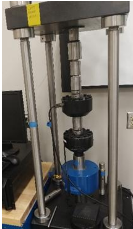
Figure 3: Picture of a Compression/Tension Machine that Does Not Replicate Field Use
