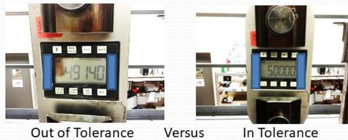
Figure 11: Tension Link Difference in output with pin size
